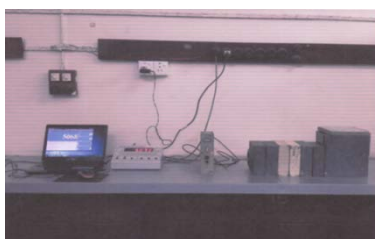
Figure 1. The operating system of NaI (Tl) detector and ST-360 radiation counter with high voltage power supply in the form of narrow beam
