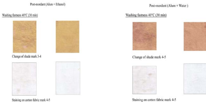
Figure 5. Washing fastness properties of dyed cotton fabric using mordant alum
