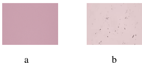
Figure 2. (a) Photomicrograph of non-irradiated film (b) Photomicrograph of irradiated film with neutron from Am (Be) source ( \times 400 )
