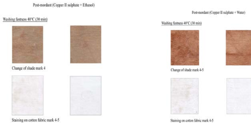
Figure 6. Washing fastness properties of dyed cotton fabric using mordant Copper (II) sulphate
