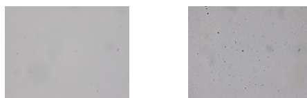
Figure 3. (a) Photomicrograph of non-irradiated glass (b) Photomicrograph of irradiated glass with neutron from Am (Be) source ( \times 400 )
