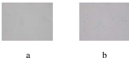
Figure 1. (a) Photomicrograph of non-irradiated mica (b) Photomicrograph of irradiated mica with neutron from Am (Be) source ( \times 400 )
